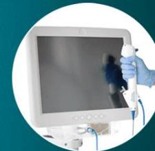
All-in-one, touch-screen PC includes the monitor, image processor and controller.
